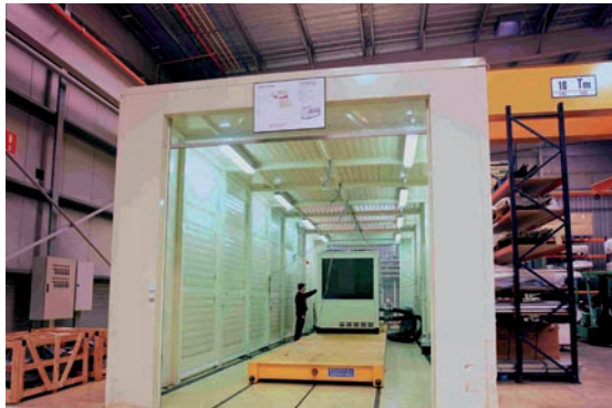
All the chillers are submitted to a Commercial Test, during which the unit is tested by simulating actual operating conditions.
